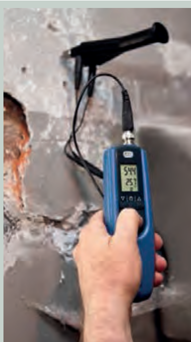
APPLICATION Measurement of plaster moisture using an M 20 electrode
