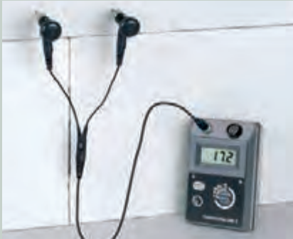
APPLICATION TIP Ideal electrode clearance: 10 cm
